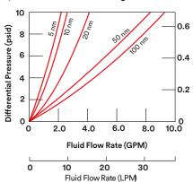
Graph 3: Typical Fluid Flow Rates @ 25° C (20" NanoSHIELD™ Cartridge - 222 connector)
