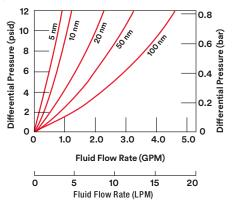
Graph 2: Typical Fluid Flow Rates @ 25° C (10" NanoSHIELD LDC™ with <sup>1</sup>/2" Flowell Connections)
