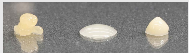
▲ Figure 5. Clarity Attachment Material (right) compared to Dentsply Sirona's SDR® flow+ (middle) and GC Aligner Connect™ (left). This image was taken 1 minute after dispensing. It shows how the Clarity Attachment Material delivers a good rheological profile that smooths out small imperfections, but does not flow enough to flow out of the tray (further evidence of this claim in Figure 3).
