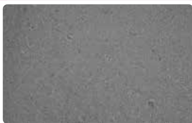
Surface of Imprint™ 4 Preliminary VPS Material shown with a Laser Scanning Microscope (objective lens with 20× magnification).
