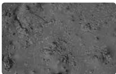
Alginate surface (Palgat™ Plus, 3M ESPE) shown with a Laser Scanning Microscope (objective lens with 20× magnification).
