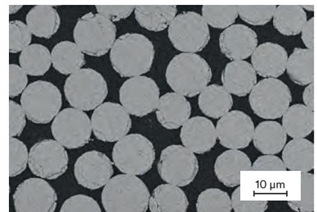
**Fig. 2:** SEM image (magnification 2kx) of a cross-section of 3M™ RelyX™ Fiber Post 3D Glass Fiber Post. Glass fibers are depicted as white spots surrounded by a composite resin matrix. Source: 3M Oral Care internal data.
