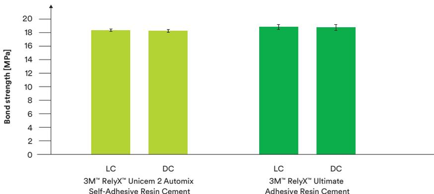
**Fig. 6:** Pull-off bond strength values of 3M™ RelyX™ Ultimate Adhesive Resin Cement and 3M™ RelyX™ Unicem 2 Automix Cement in comparison. Both materials show same performance in light-cure (LC) and dark-cure (DC) mode. Source: Peez et al.<sup>2</sup>
