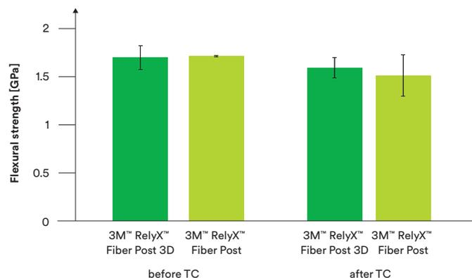
**Fig. 5: One-point flexural strength testing before and after thermocycling (TC), 10,000 cycles, 5°C/55°C, dwell time 30 s, change time 8 s.** Source: 3M Oral Care internal data. Data available upon request. See last page for contact information.
