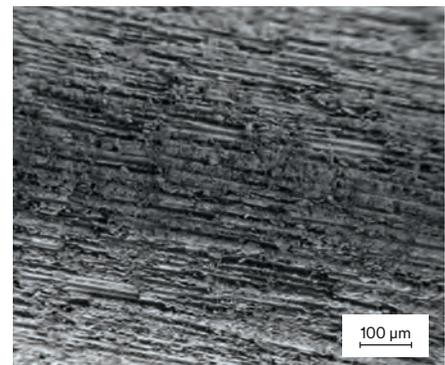
**Fig. 7:** Surface of 3M™ RelyX™ Fiber Post 3D Glass Fiber Post (SEM, 200x magnification). Source: Peez et al.<sup>2</sup>
