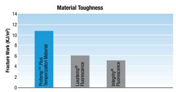
In a test measuring material toughness, Protemp<sup>™</sup> Plus Temporization Material showed greater resistance to fracture than other temporization materials. Source: V. Babcic, R. Perry and G. Kugel, Tufts University, Boston, MA, U.S.A., AADR 2008, #0371
