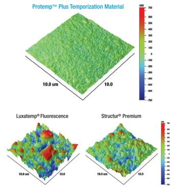
Surface topology of Protemp<sup>™</sup> Plus and other temporization materials after removing the inhibition layer with alcohol and no further polishing.
