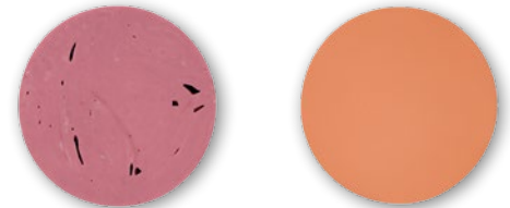
Fig. 1: Hand-mixed putty (left) compared to an automatically mixed putty material out of the Pentamix™ System from 3M ESPE (right). The automatically mixed impression material is homogeneously mixed and does not show any voids.
