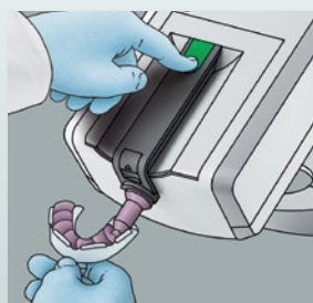
7. Press the green start button to fill the impression tray or elastomer syringe.
