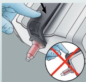
6. Close the latch with an audible click.
