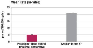
**In-vitro wear:** Wear rates were determined using a 3-body, in-vitro test. Dimensional loss during the 200,000 cycle test was measured every 40,000 cycles and the wear rates were calculated using linear regression. Paradigm Nano Hybrid restorative exhibited less wear than Gradia Direct X.
