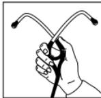
To increase spring tension, grasp the headset with one hand where the eartubes enter the plastic tubing and squeeze until the plastic tubing on one eartube touches the other. Repeat as necessary.
