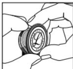
To attach the rim/diaphragm assembly to the chestpiece, engage the groove of the rim (with the diaphragm attached) around the chestpiece at one point and hold it in place with your thumbs.
