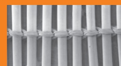
Hollow fiber membrane array
