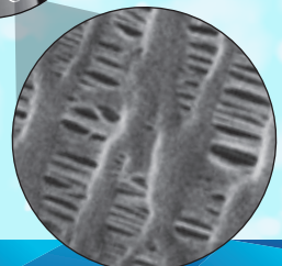
Hydrophobic membrane with pores approx. 0.03 μm
