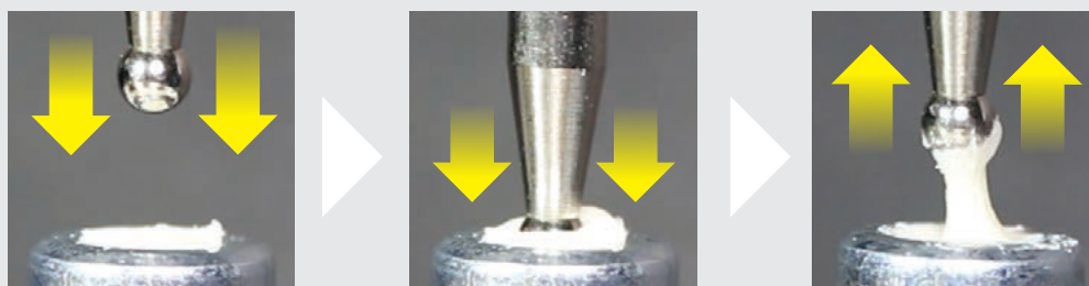
Figure 6: Test method: dipping of the plunger into the mixed paste and withdrawal immediately afterwards.
