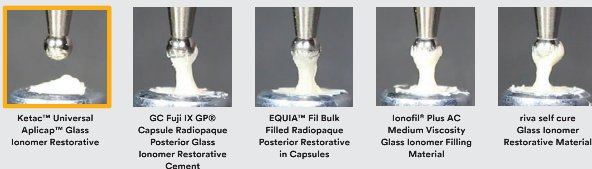
Figure 7: Stickiness test: different materials after withdrawal of the steel ball. Source: 3M internal data
