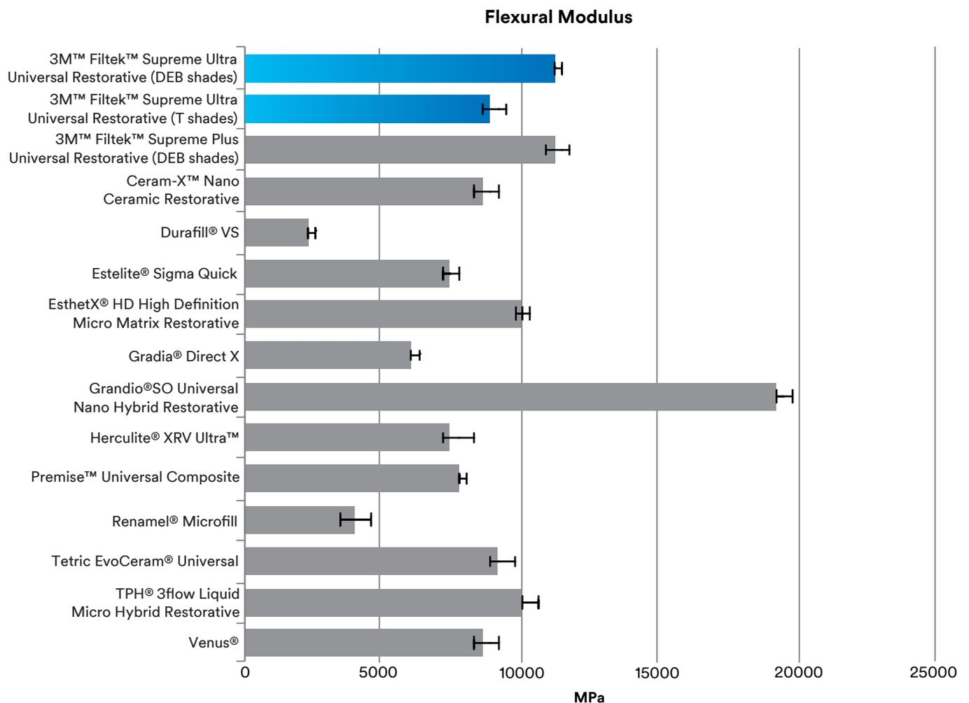
Flexural modulus. Source: 3M internal data
