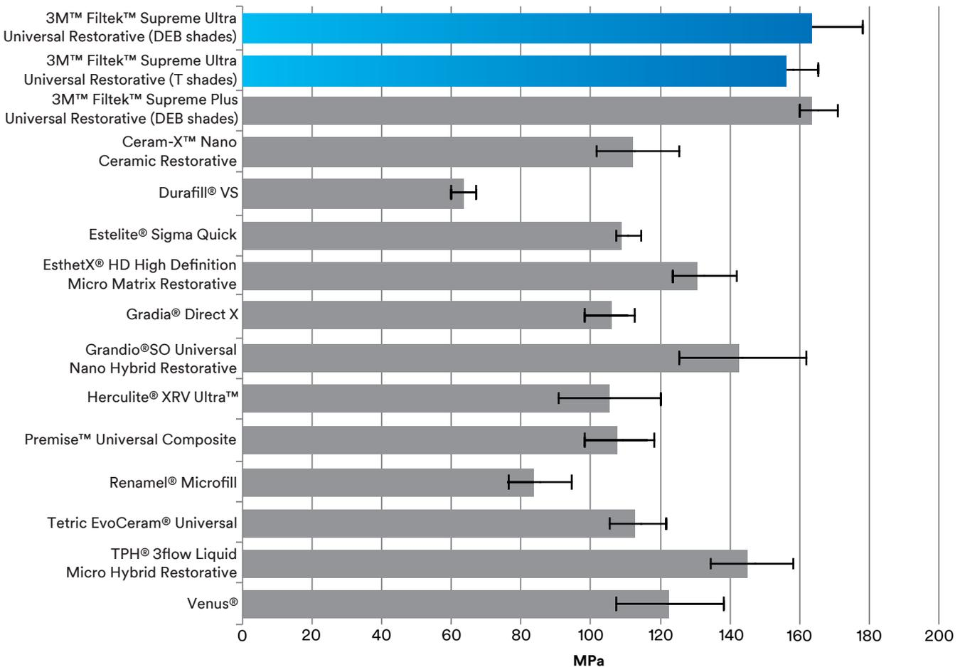
Flexural strength. Source: 3M internal data
