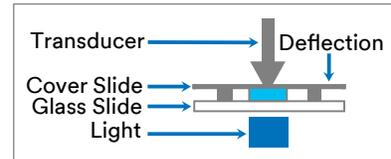
In this test, samples were exposed for 60 seconds to a 3M™ Visilux™ 2 Visible Light Curing Unit. The final shrinkage was recorded 4 minutes after the end of light exposure.
