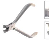
Unitek<sup>™</sup> Lingual Distal End Cutter Used for a wide range of wire sizes. It features long handles and a narrow design, with cutting tips made of Tungsten Carbide for durability. A clean square end cut reduces deburring, and the safety hold feature secures the loose wire after the archwire is cut. Minimum wire cutting capacity: .012" (.30 mm)
