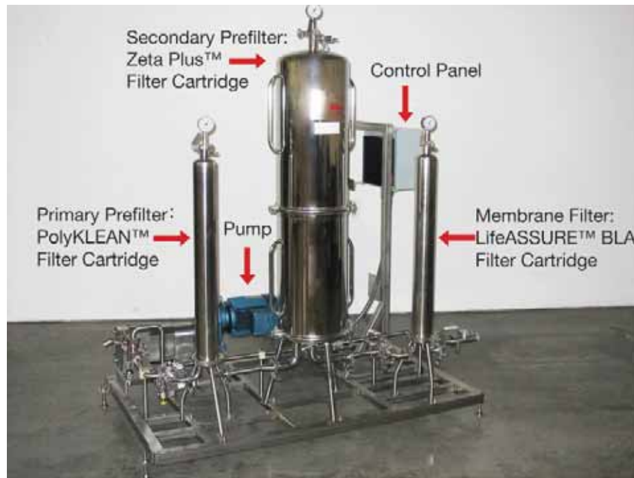
Figure 9. Three-stage filtration system for anti-browning solution
