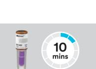
Cool 4 After completion of cycle, retrieve PCD, remove BI and allow BI to cool 10 minutes prior to activation.
