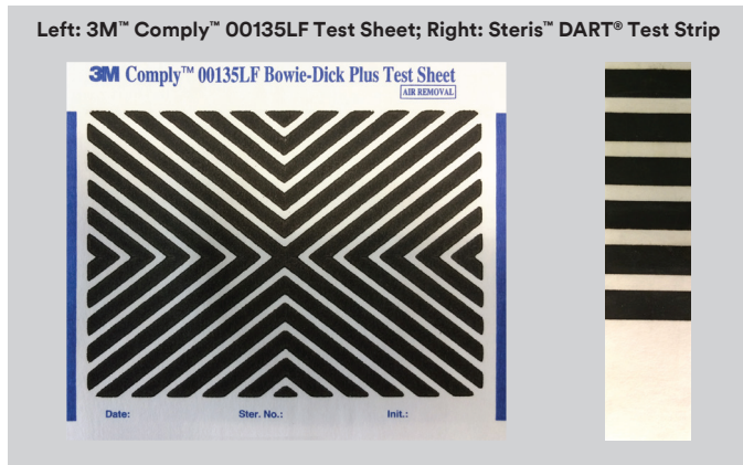
Figure 3: Bowie-Dick Test Results — Control Cycle (No Air Leak)
