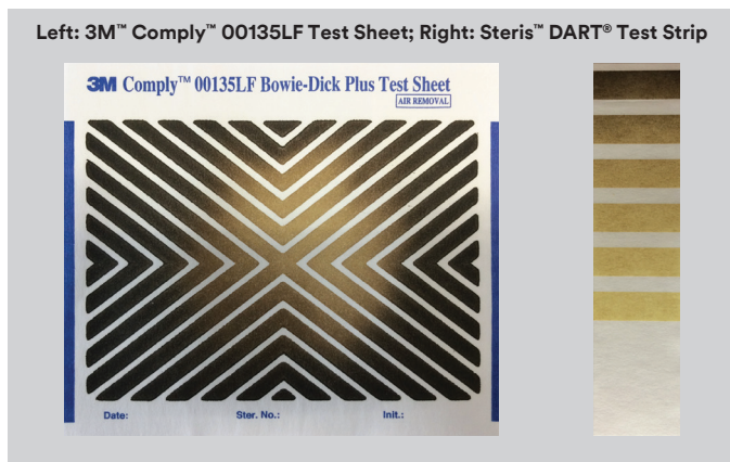
Figure 4: Bowie-Dick Test Results — Air Leak Cycle
