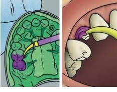
Syringe wash material around the preparation and into the preliminary impression.
