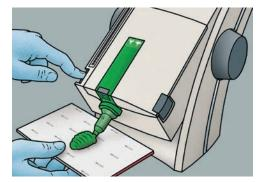
When using new foil bags, start mixing and extrude a small amount until paste is homogeneous in color. Discard.
