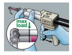
Hold firmly in place while filling. Leave mixing tip in angled position; do not fold open. Do not fill syringe past the maximum fill line.
