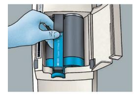
Insert the loaded cartridge into the 3M<sup>™</sup> Pentamix<sup>™</sup> Automatic Mixing Unit.
