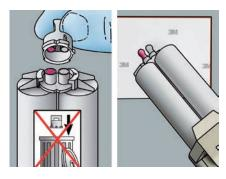
Remove the cartridge cap. Bleed a small amount of material from the cartridge onto mixing pad and discard.
