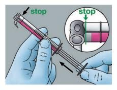
Replace plunger in the syringe, pushing paste no further than to the joint of the mixing tip.
