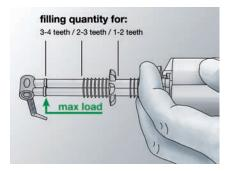
The content of an intra-oral syringe is sufficient for syringing about 2-4 preparations, depending on the quantity applied around each unit.
