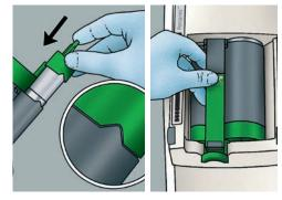
Place the 3M<sup>™</sup> Penta<sup>™</sup> foil bags into the designated 3M<sup>™</sup> Penta<sup>™</sup> cartridge. Insert the loaded cartridge into the 3M<sup>™</sup> Pentamix<sup>™</sup> 3 Automatic Mixing Unit.
