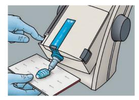
When using new foil bags, start mixing and extrude a small amount until paste is homogeneous in color. Discard.
