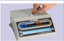
Hold BI by cap and use "crusher well" to crush the media ampoule.
