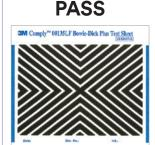
Indicator ink circle on Early Warning Test Sheet is lighter than the color standard but Bowie-Dick Test Sheet shows a uniform color change to dark brown/black. Sterilizer can be used but sterilizer maintenance should be scheduled.
