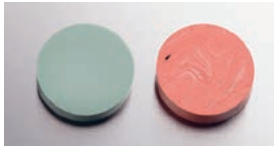
Fig. 27: Superior mixing quality of automatically mixed 3M™ Express™ 2 Penta™ Putty VPS Material using the 3M™ Pentamix™ Mixing Unit (left) compared to a putty mixed by hand (right, 3M™ Express™ STD Putty).
