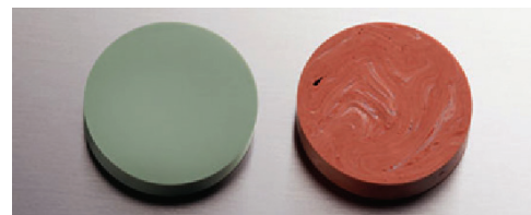
Fig. 6b: Superior mixing quality of 3M™ Express™ XT Penta™ Putty Material automatically mixed with the 3M™ Pentamix™ 3 Mixing Unit (left) compared with a hand-mixed putty (right, 3M™ Express™ STD Putty).
