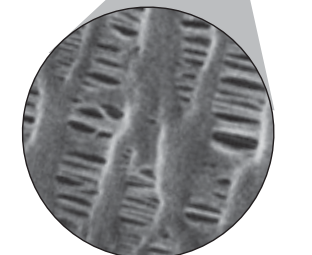
Hydrophobic membrane with pores approx. 0.03 μm
