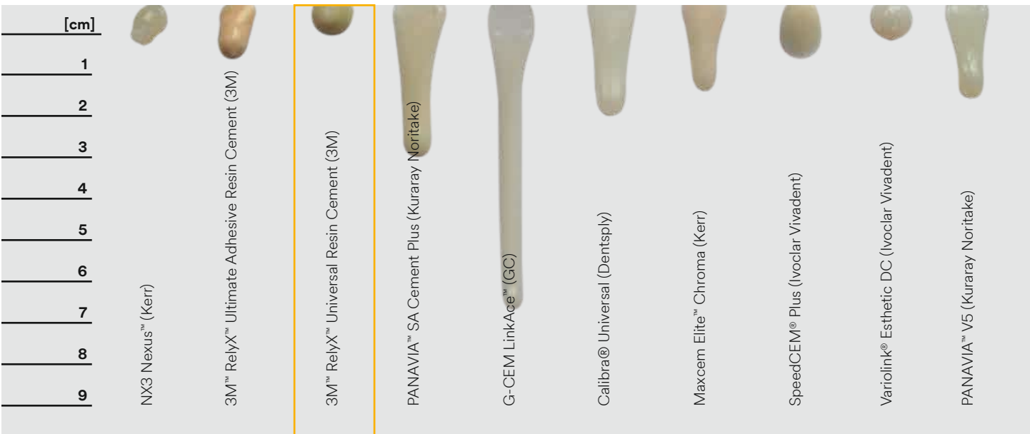
Fig. 2: To compare the flow properties, equal amounts of each cement were applied on a pad which was stored upright at 36°C/96.8°C for 2 minutes before the cement was light-cured. Source: 3M internal data
