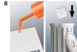
Do not use high pressure. Check mixer position (image 7) if extrusion force is high.
