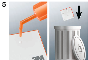
Discard a small amount of cement.
