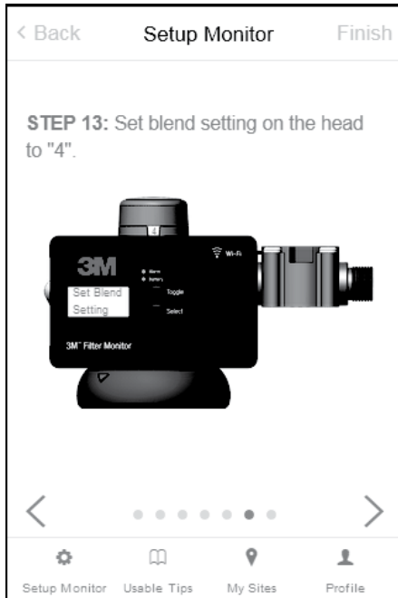
Wi-Fi Monitor Setup - STEP 13 Set blend setting on the head as per APP instructions.
