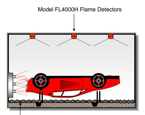
NFPA 33 regulation requires optical flame detection system shutdown upon detection of a fire in electrostatic paint spray booths, used in major automobile plants.
