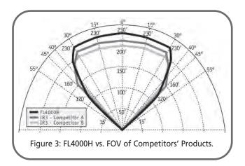
comparison of the FL4000H vs. competitive technologies is presented in Figure 3 above for the high sensitivity setting. The FL4000H provides a longer range of flame detection (230 feet) while maintaining a wide field of view. Table 1 shows the FL4000H's field of view at various distances. The FL4000H offers the largest angular coverage at the longest detection distance amongst flame detectors within the marketplace.
