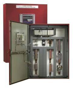
Wall mounted NEMA 12 enclosure. Customer connections made at rail mounted "swing link" terminal blocks organized by input/output type.
