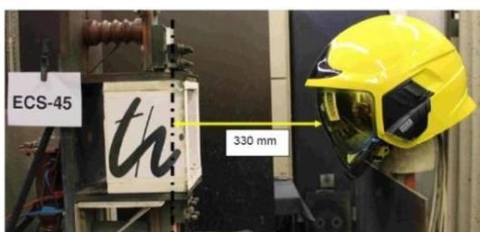
Figure 2: Test set-up with helmet visor combination
