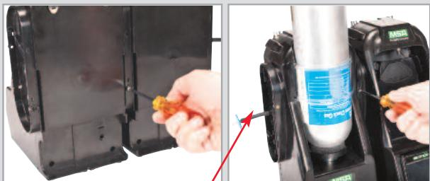
If using MSA cylinder holders, left-most cylinder holder should have fresh air filter attached to top port.
