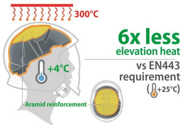
The aramid layer on the top of the impact liner also provides a **higher thermal performance**. The thermal protection it delivers proves to be a major competitive advantage too, as it is perceivable by users in hot trainings or real fire situations. In many real fire testing situations, it succeeded in negating any heat breakthrough longer than any other helmet.
