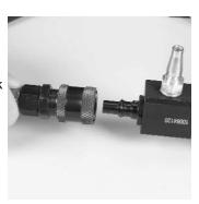
Disconnect the test manifold assembly from the first stage intermediate pressure hose.
