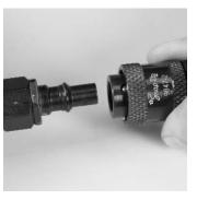
Connect test manifold assembly to first stage intermediate pressure hose.
