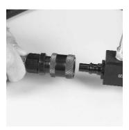
Connect the test manifold assembly to PosiChek<sup>3</sup> intermediate pressure hose.
