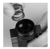
Removing the Seat and Seat O-Rings
