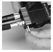
Pull the hose firmly to remove it from the regulator body.
