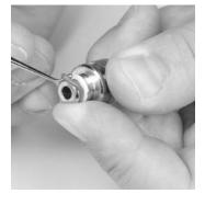
4. Install the high pressure gauge hose into the high pressure gauge port.
