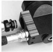
5. Leak test the regulator.
