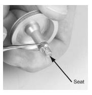
4. Use the o-ring removal tool to remove the piston head o-ring.
