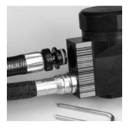
3. Use the o-ring removal tool to remove the o-ring.
