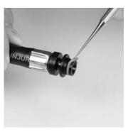
5. Pull the hose firmly to remove it from the regulator body.
