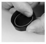
**Note:** Ensure that the o-ring is completely seated.
