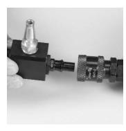
Connect the AirHawk II hose to test manifold assembly.
