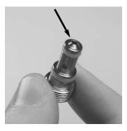
2. Use the o-ring removal tool to remove the top seat oring.
