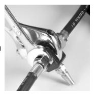
4. Connect the test manifold assembly to PosiChek<sup>3</sup> intermediate pressure hose.
