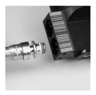
6. Use the o-ring removal tool to remove the o-ring and back-up ring from the hose fitting.
