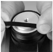
**Note:** Be careful not to damage the seal ring sealing surfaces.
