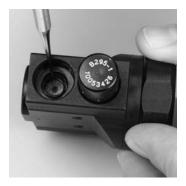
Note: Do not lubricate the filter o-ring.
