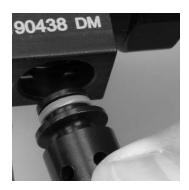
Install the high pressure Audi-Larm hose into the high pressure supply port.
