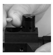
2. Install the filter o-ring into port and seat it against the filter.
