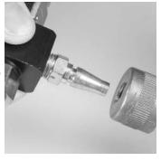
Connecting the Test Manifold Assembly, Quick-Connect and ExtendAire Hoses
