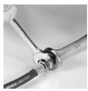
Screw the test manifold assembly onto first stage intermediate pressure hose until tight.
