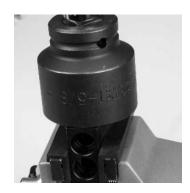
Installing the Pressure Relief Valve
