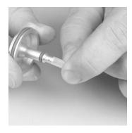
9. Install the piston into the regulator body.
