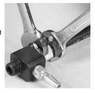
Screw the AiHawk II hose onto test manifold assembly until tight.
