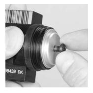
2. Pull gently on the mounting screw to extract the piston from the regulator body.
