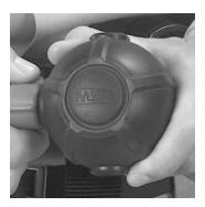
Reach behind and open the cylinder valve fully. Listen for the alarm to sound briefly.
