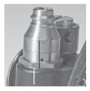
...or across the joint where the coupling attaches to the air mask, remove the air mask from service until a replacement coupling is installed. If the line does line up, the coupling is sufficiently tight and the air mask may be returned to service.
