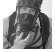
Push the release buttons and pull regulator down and out of facepiece adapter.
