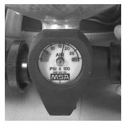
As the pressure rises from 50 to 200 psig, the alarm sounds automatically, indicating that the alarm is functional.
