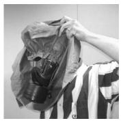
5. Carefully tuck the elastic lens opening of the hood around the back of the facepiece lens rings, component housing assembly, and applicable accessory. The rain shield of the hood should be uniformly over the upper lens ring of the facepiece. The elastic lens
