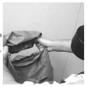
**Note:** If using the ClearCommand voice amplifier accessory with the RI Connection, place the cable through the lens opening of the hood and move the ear phone toward the lens of the facepiece. This will allow the lens opening of the hood to slide over the ear phone and amplifier.
