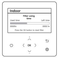
After cleaning and reassembling the air filter, be sure to reset the filter-cleaning reminder as follows:
