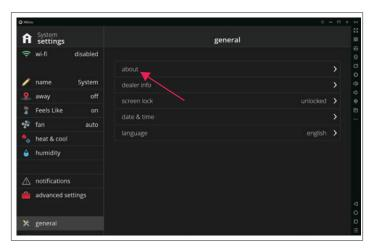
Got to the thermostat section and verify both thermostat and smart hub control software revisions. Both will need to be version 03.40.xxx or higher.
