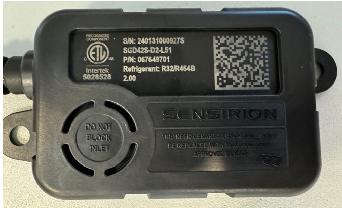
FIGURE 11. Example of Clear, Unobstructed Sensor Inlet
