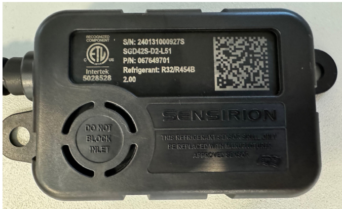
FIGURE 13. Example of Clear, Unobstructed Sensor Inlet
