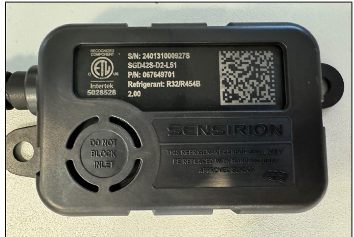
FIGURE 24. Example of Clear, Unobstructed Sensor Inlet
