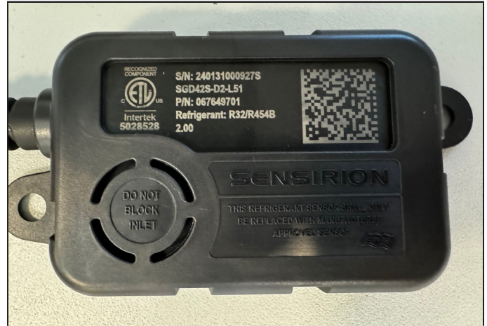
FIGURE 34. Example of Clear, Unobstructed Sensor Inlet
