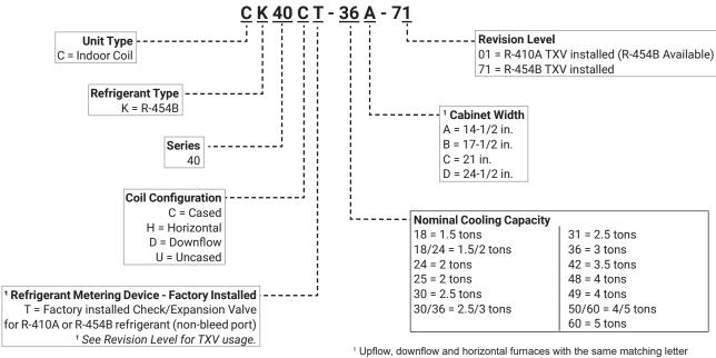
designation physically match upflow, downflow and horizontal indoor coils. Uncased upflow coils have different widths, but will fit the corresponding furnace cabinet.
