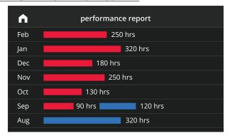
Displays the number of hours each month the system has been operating in heating mode (red) or cooling mode (blue) in an easy-to-read graph.
