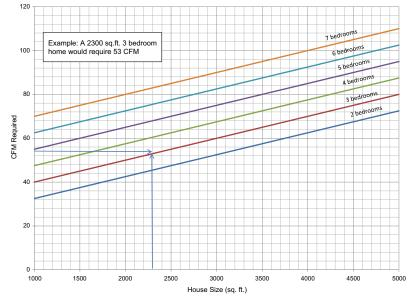
Step 2 - Determine How Much Ventilation Air the System will Deliver
