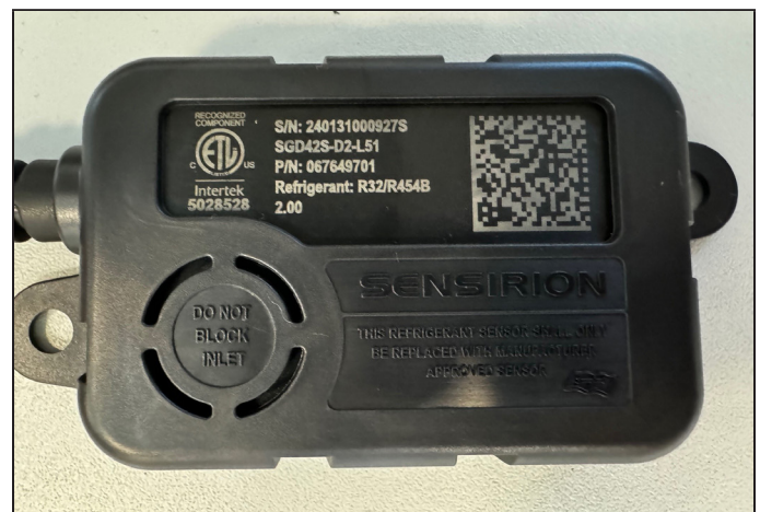
FIGURE 33. Example of Clear, Unobstructed Sensor Inlet
