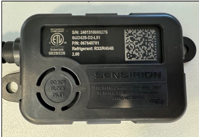
FIGURE 35. Example of Clear, Unobstructed Sensor Inlet
