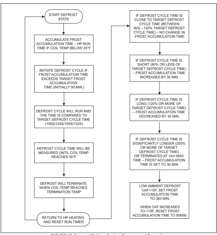
FIGURE 35. Demand Defrost Cycle - Sequence of Operation
