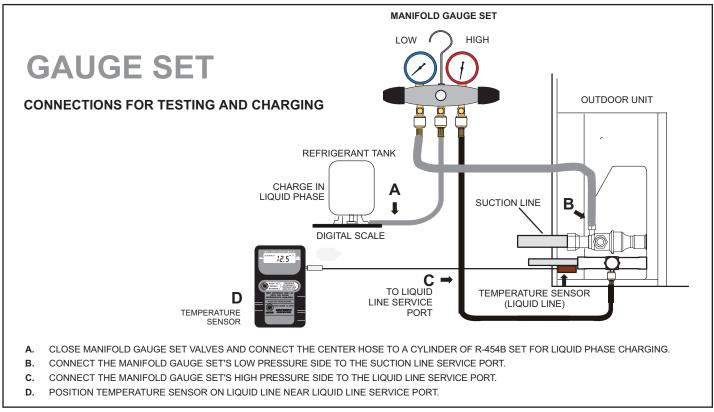
FIGURE 55. Gauge Set Connections
