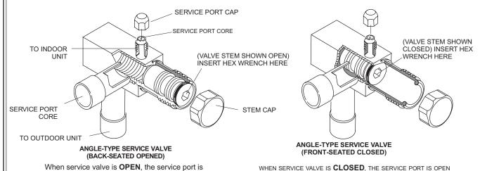
When service valve is **OPEN**, the service port is open to linE set, indoor and outdoor unit.
