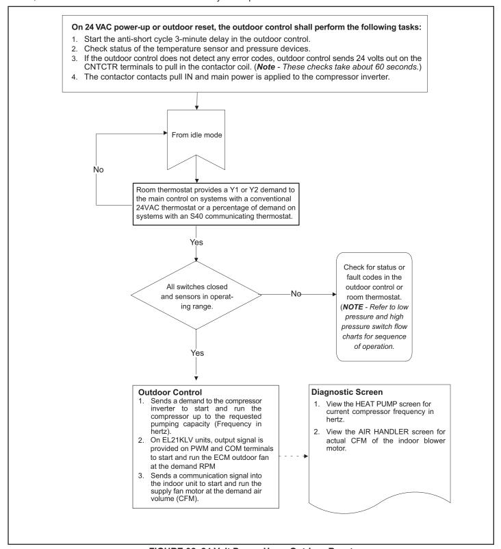
FIGURE 32. 24 Volt Power-Up or Outdoor Reset
