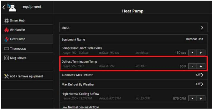
FIGURE 19. Defrost Termination Temp Setting in the S40 Thermostat
