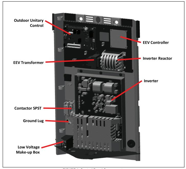
**FIGURE 1. Control Panel Components**
