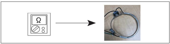
FIGURE 43. Checking Belly-Band Crankcase Heater
