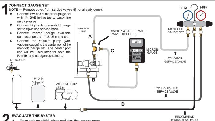
Open both manifold valves and start the vacuum pump.
