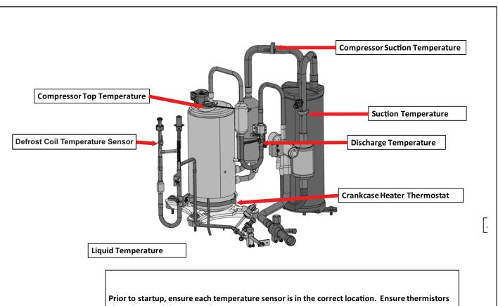
clipped on to piping are not loose.
