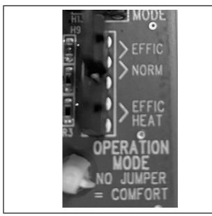
FIGURE 51. Operation Mode Jumper
