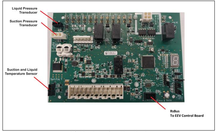
FIGURE 23. Unitary Control Board Detail
