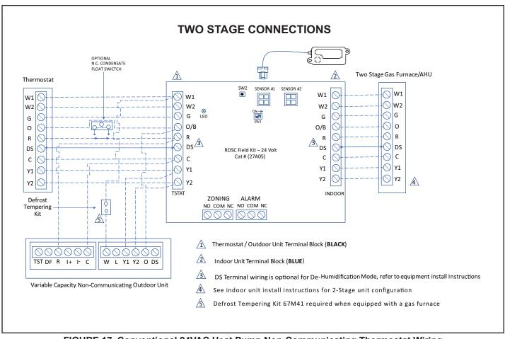
FIGURE 17. Conventional 24VAC Heat Pump Non-Communicating Thermostat Wiring
