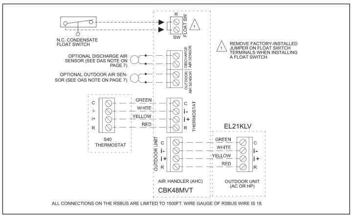
FIGURE 16. Communicating System Wiring Diagram - EL21KLV with CBK48MVT Communicating Air Handler with Integral RDS Control
