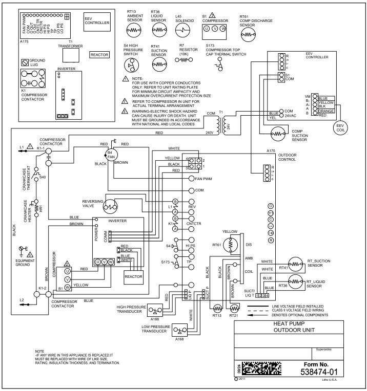
FIGURE 30. Typical Unit Wiring (EL21KLV)
