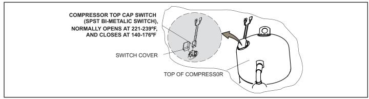
FIGURE 46. Top Cap Thermal Sensor Switch
