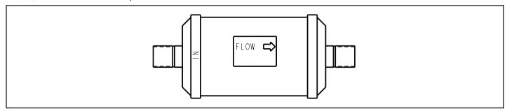
FIGURE 45. Suction line filter drier
