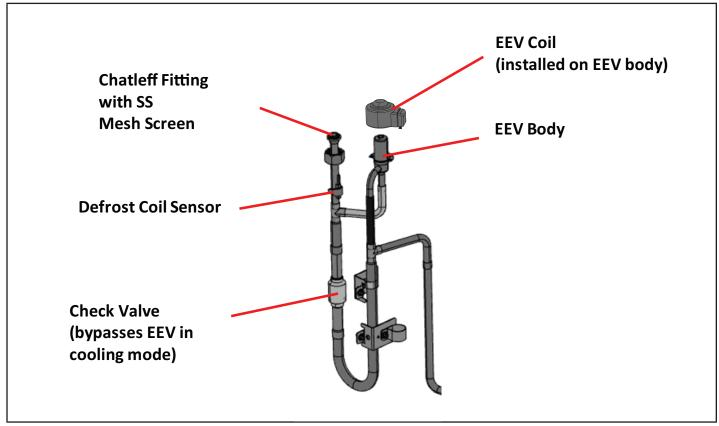
FIGURE 21. EEV Piping Assembly
