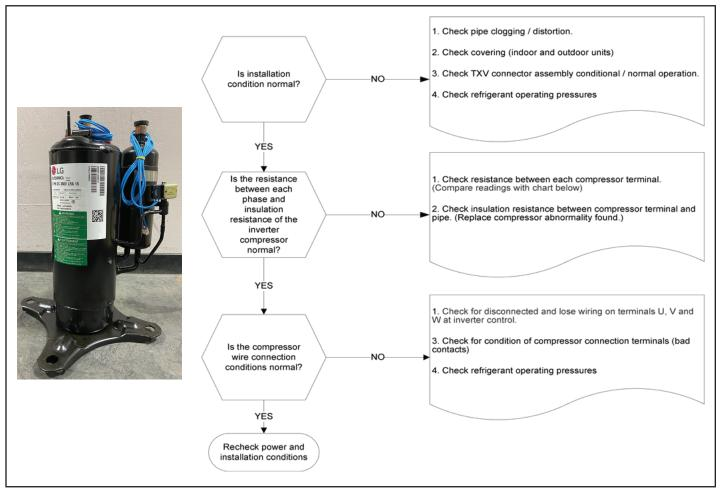
FIGURE 41. Compressor Operation, Checkout and Status/Error Codes
