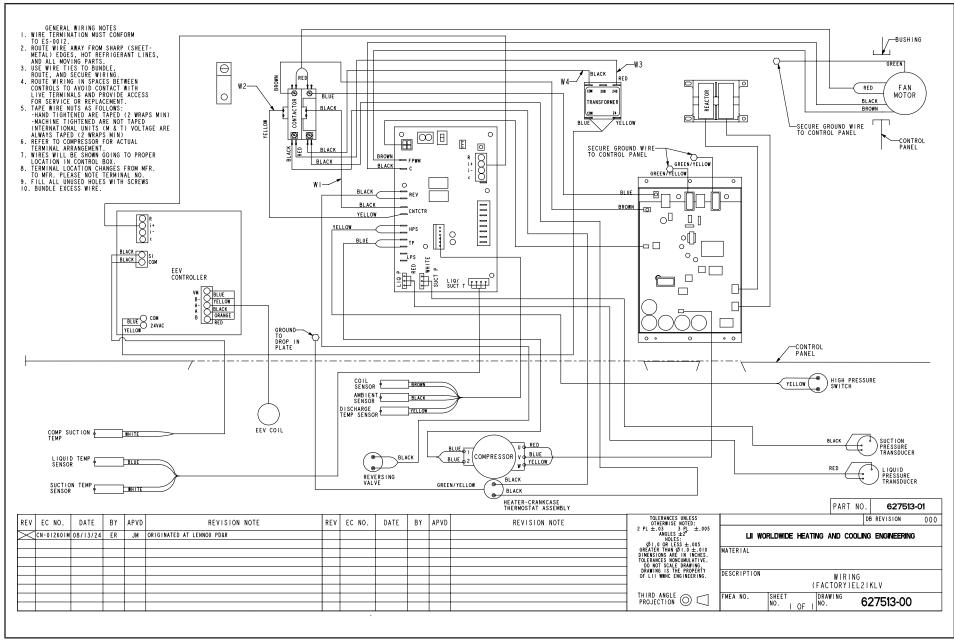
FIGURE 31. Typical Unit Wiring (EL21KLV)
