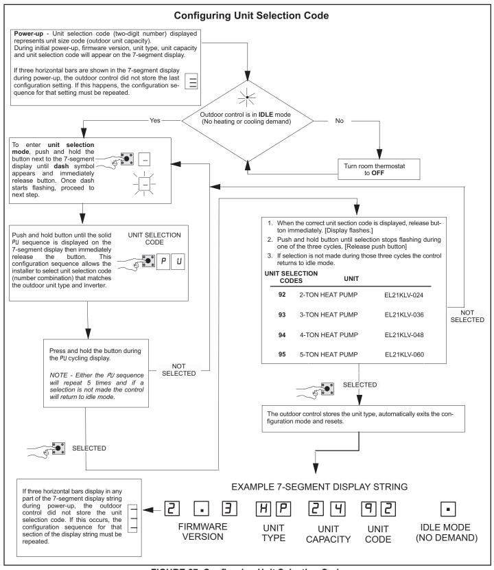
FIGURE 27. Configuring Unit Selection Code
