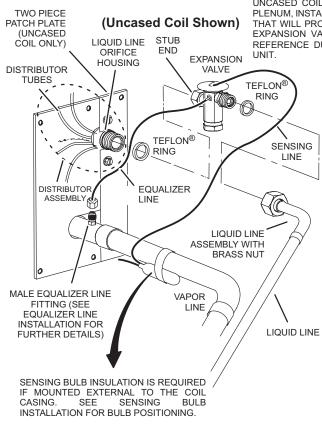
THE EXPANSION VALVE UNIT CAN BE INSTALLED INTERNAL OR EXTERNAL TO THE INDOOR COIL. IN APPLICATIONS WHERE AN UNCASED COIL IS BEING INSTALLED IN A FIELD-PROVIDED PLENUM, INSTALL THE CHECK EXPANSION VALVE IN A MANNER THAT WILL PROVIDE ACCESS FOR FIELD SERVICING OF THE EXPANSION VALVE. REFER TO BELOW ILLUSTRATION FOR REFERENCE DURING INSTALLATION OF EXPANSION VALVE
