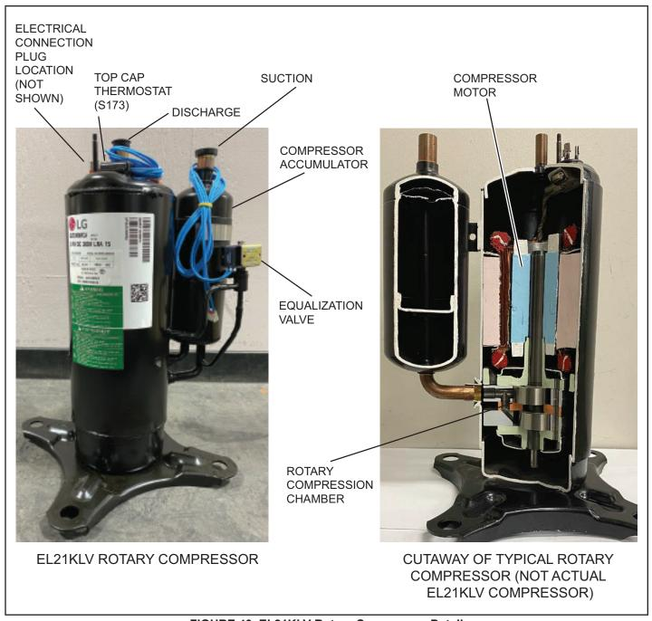
FIGURE 40. EL21KLV Rotary Compressor Detail
