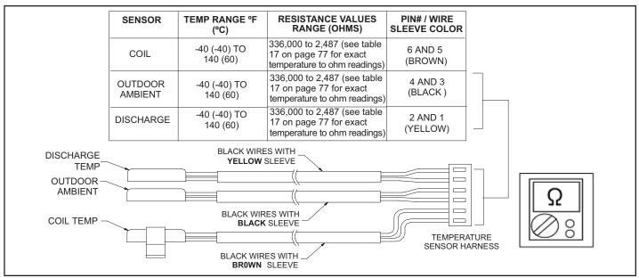
FIGURE 52. Temperature Sensor Specification
