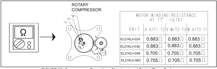
FIGURE 39. Compressor Operation, Checkout and Status/Error Codes
