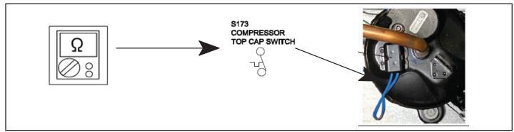
FIGURE 47. Verifying Top Cap Thermal Sensor Switch
