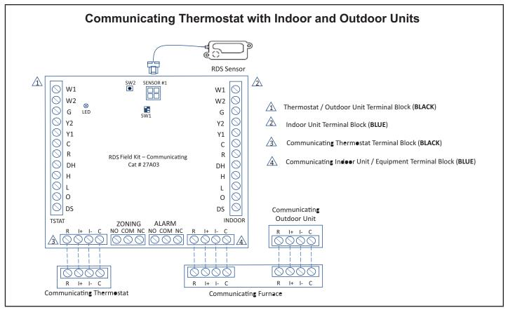
FIGURE 15. Communicating System Wiring Connections
