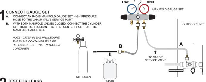
**TEST FOR LEAKS**
