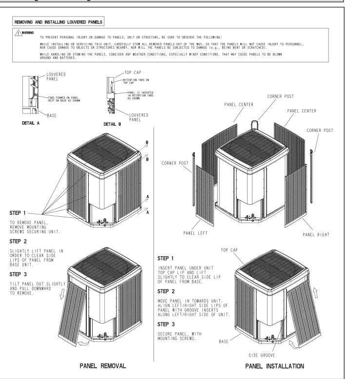
FIGURE 7. Removing and Installing Panels
