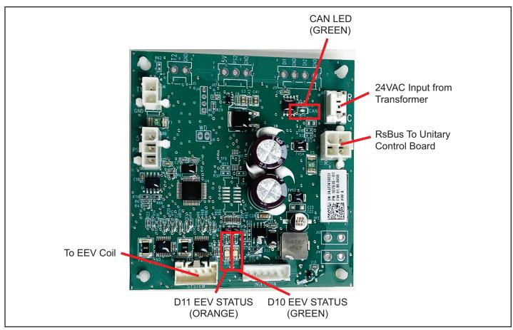
FIGURE 22. EEV Control Board Detail
