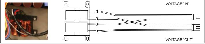
FIGURE 48. EL21KLVS/E18XCV Reactor
