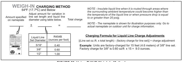
FIGURE 58. Using R454B Weigh-In Method
