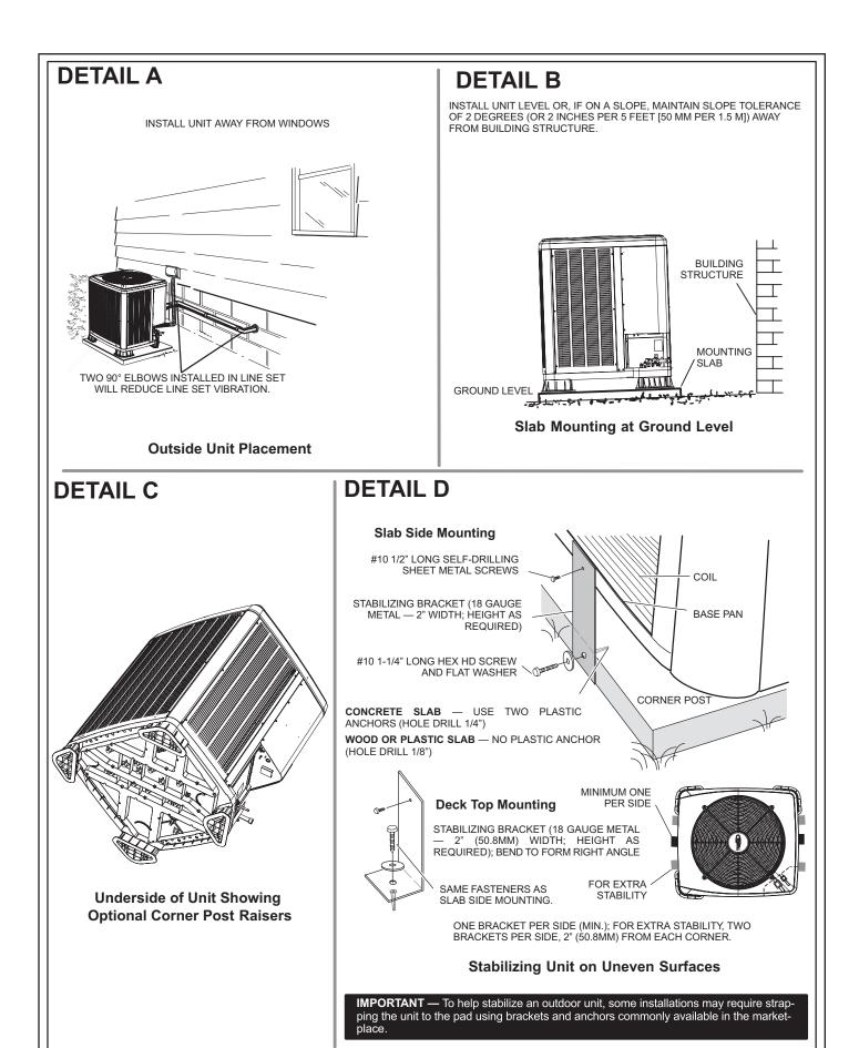
FIGURE 6. Placement and Slab Mounting
