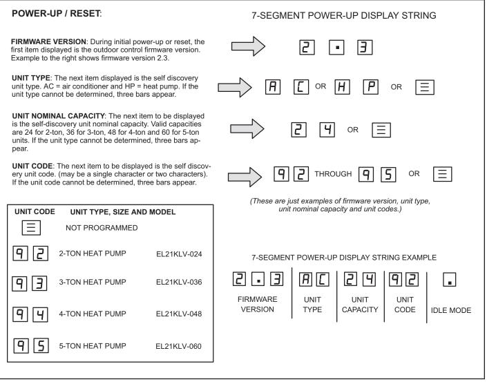
FIGURE 24. Outdoor Control 7-Segment Unit Status Displays
