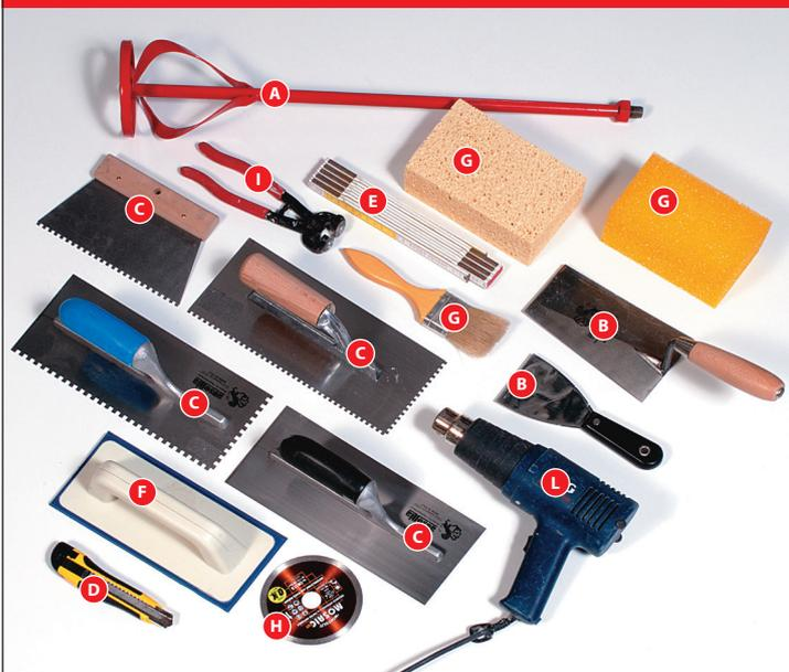
**EQUIPMENT** (A) Helicoidal whisk to mix binder and sealer (B) Stainless steel squeegees and trowels (C) Smooth squeegee, stainless steel square tooth mm 3 and mm 5 (D) Cutter (E) Measuring set (metre, pencils, ruler) (F) Rubber plasterer's trowel to flatten and plaster sheets (G) Cellulose sponges set fit for cleaning epoxy materials (H) Continuous gear diamond lapping wheel placed on angular sanding machine (I) Pincer for manual cutting fit for glass (L) Fan for adhesive film removal.
