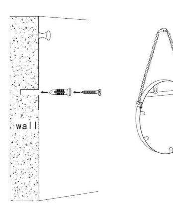
Mark three holes on wall. The distance between the two holes must match the distance on back of the unit.
