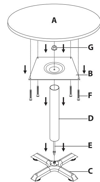
**Assembly Notes:**During assembly, hand tighten screws only. When all screws are in place, you may then tighten all screws completely.
