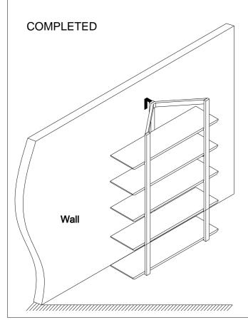
Due to the various wall construction methods, It is up to a professional installer to secure the Nylon Tape(M) to the wall with the proper fasteners and/or anchors as required by the wall construction at the desired mounting location.
